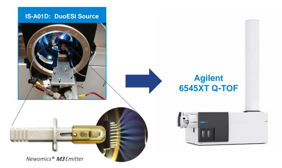
Interface between Newomics DuoESI source with Agilent 6545XT Q-TOF mass spectrometer. The DuoESI source has interchangeable interface modules for microflow LC-MS and nanoflow LC-MS applications, respectively. Shown here is the microflow module only.
